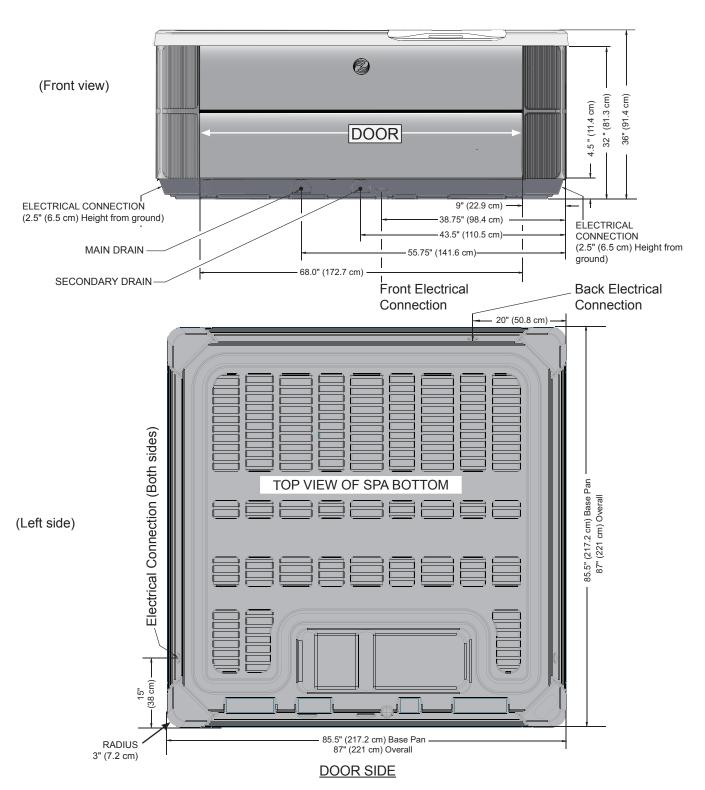
**NOTE: WATKINS WELLNESS** requires that the **ARIA** be installed on a minimum 10 cm (4") thick reinforced concrete pad or a deck that is able to withstand more than 565 kg/m² (115 lbs. per square foot).
