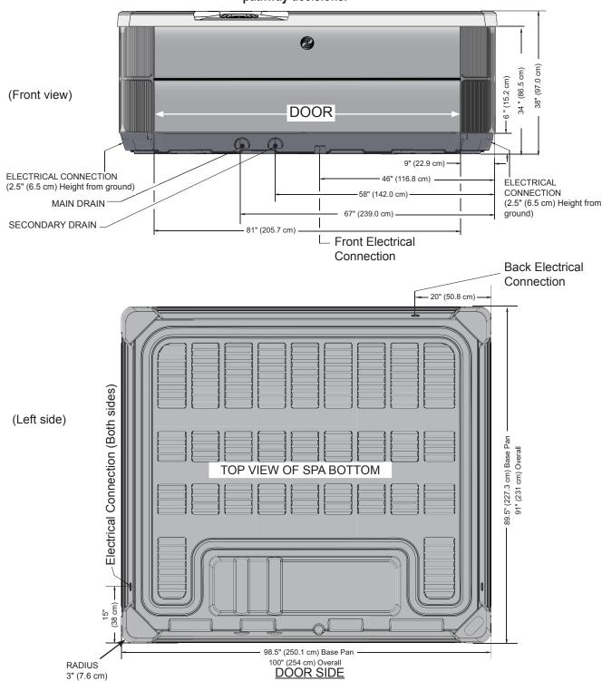
**NOTE: WATKINS WELLNESS** requires that the **ENVOY** be installed on a minimum 10 cm (4") thick reinforced concrete pad or a deck that is able to withstand more than 565 kg/m² (115 lbs. per square foot).
