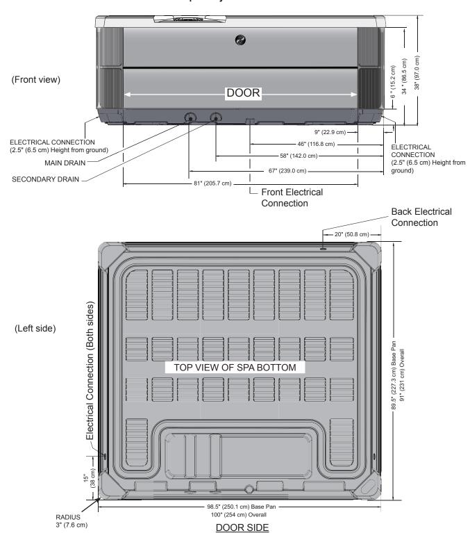
**NOTE: WATKINS WELLNESS** requires that the **GRANDEE** be installed on a minimum 10 cm (4") thick reinforced concrete pad or a deck that is able to withstand more than 555 kg/m² (125 lbs. per square foot).
