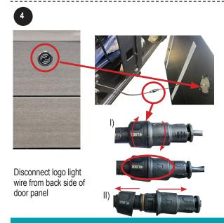
Using both hands grab wire on each side of connector and pull away from connector.
