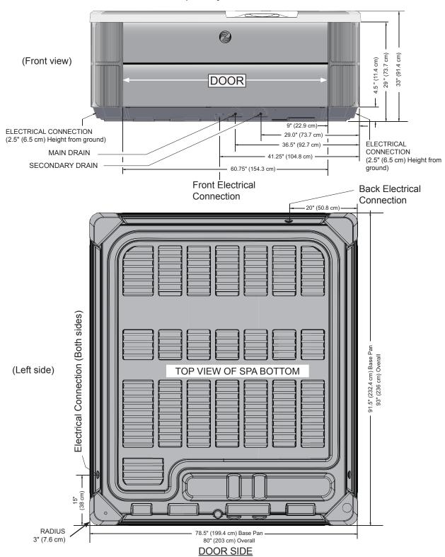
**NOTE: WATKINS WELLNESS** requires that the **SOVEREIGN** be installed on a minimum 10 cm (4") thick reinforced concrete pad or a deck that is able to withstand more than 530 kg/m² (110 lbs. per square foot).
