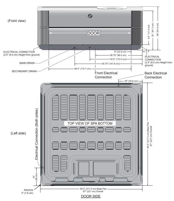
**NOTE: WATKINS WELLNESS** requires that the **VANGUARD** be installed on a minimum 10 cm (4") thick reinforced concrete pad or a deck that is able to withstand more than 565 kg/m<sup>2</sup> (115 lbs. per square foot).
