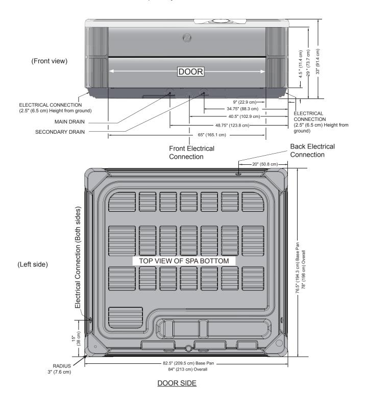
**NOTE: WATKINS WELLNESS** requires that the **PRODIGY** be installed on a minimum 10 cm (4") thick reinforced concrete pad or a deck that is able to withstand more than 595 kg/m $^2$  (125 lbs. per square foot).
